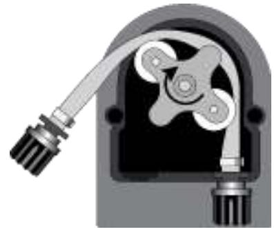
Completely release the left connector, holding it taut towards the outside, and turn the roller in the direction of the circular arrow so that the hose is freed up to the right connector.
