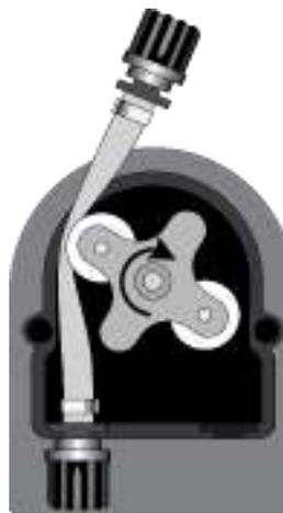
Insert the left connector into the relative housing and pass the hose under the roller's guide. Turn the roller in the direction of the circular arrow, simultaneously accompanying the hose into the pump's head, until the right connector is reached.
