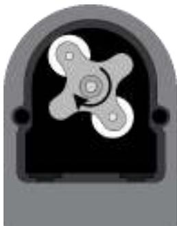
Position the roller at 7h05, turning it in the direction of the circular arrow.
