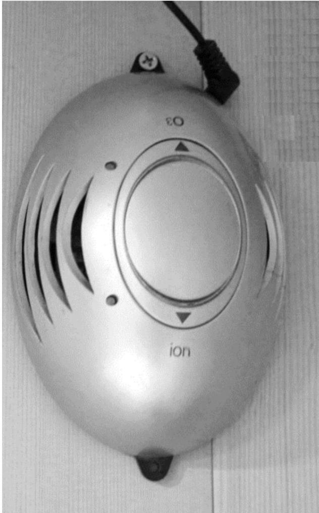
The ION button is used to switch on the ionizer. After pressing, the control diode lights up - green.
